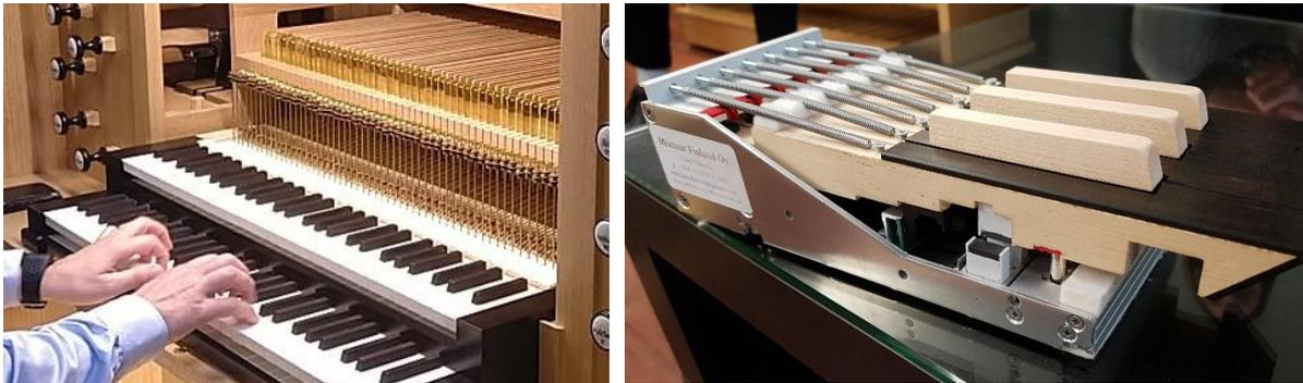
Picture 2a and 2b: Mechanical pipe organ (Suomenlinna church) and UHT™ virtual organ keys with contactor switches, magnets and springs.
